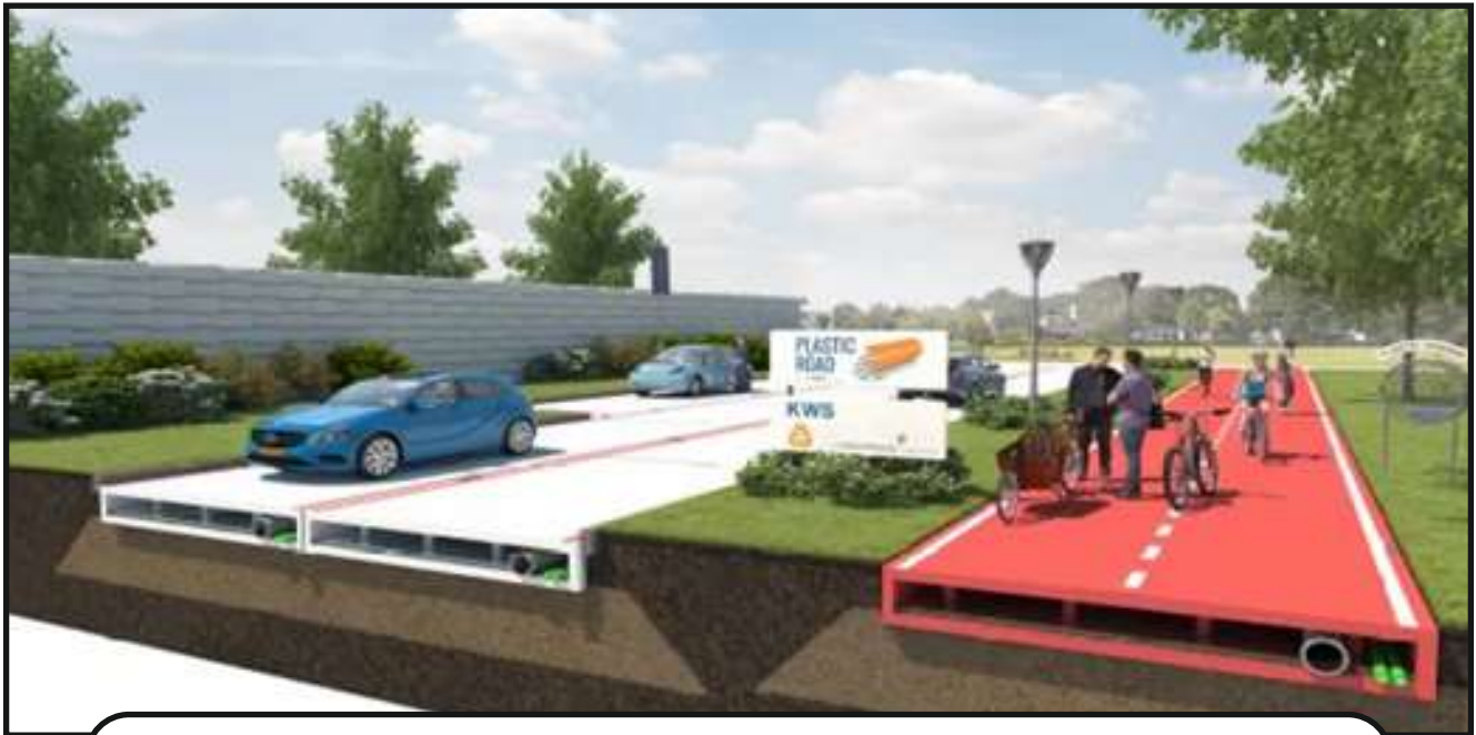
Conceptual Photo of Road Construction with Plastic Board
